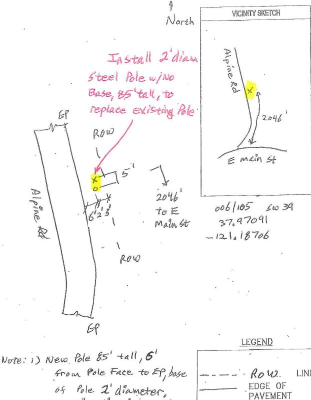
of Pole 2' diameter. 2) Install 36"x36" x12" control box on Field side of pole. LINE
